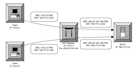
Figure 1.2: A complex NAT gateway, performing port-address translation. Notice that the gateway modifies the *source* IP address and port of each the packet.
